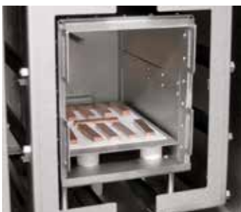
Heat treatment of copper bars under hydrogen in VHT 8/16-MO
