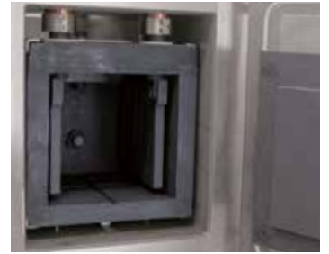
Graphite heating chamber
