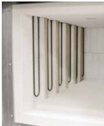
Protection of heating elements against mechanical damage
