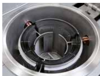
Cylindrical retort with tungsten heating
