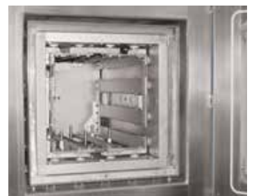
Tungsten heating chamber
