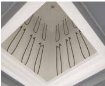
Heating elements arranged one above the other for tall structures
