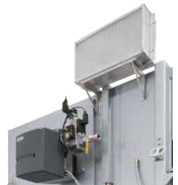
Direct gas-firing at a chamber dryer
